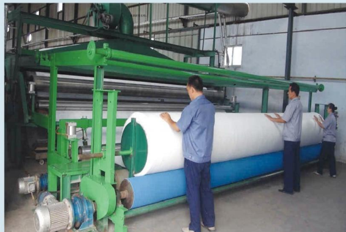
Singeing Geotextile Production Line
